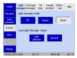
Fig. 4-85 Microscope -> Settings -> Extras -> Light manager
