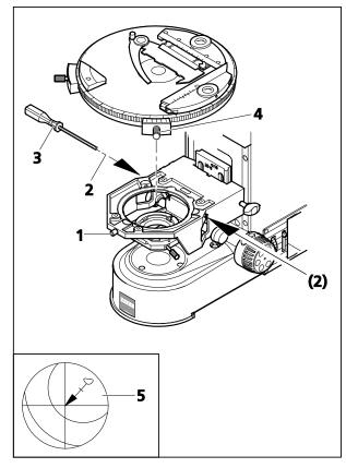
Fig. 3-57 Centering rotary stage Pol
