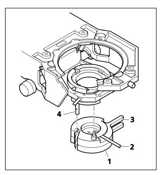
Fig. 4-3 Polarizer for transmitted light
