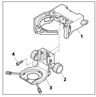
Fig. 3-18 Attaching the condenser carrier to the stage carrier
