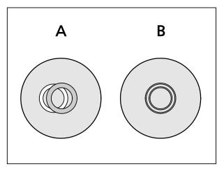
Fig. 4-119 Centering the phase stop (bright ring in condenser) to the phase ring (dark ring in objective)
