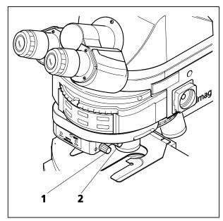
Fig. 4-121 Motorized four-position modulator turret for transmitted-light DIC
