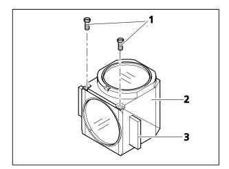
Fig. 3-25 Changing the beam splitter
