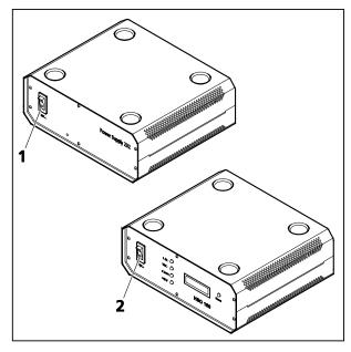
Fig. 4-10 Switching motorized microscope and HBO 100 illuminator on/off
