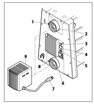
Fig. 3-35 Attaching the HAL 100 halogen illuminator
