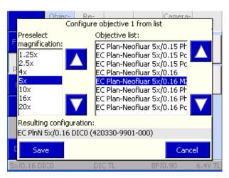
Fig. 4-58 Configuring of objective from list
