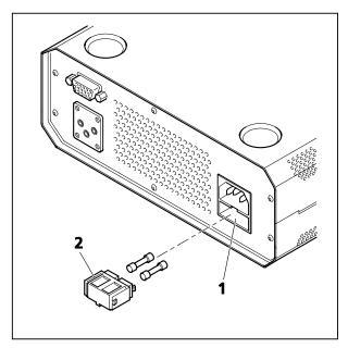
Fig. 5-2 Changing fuses on the power supply
