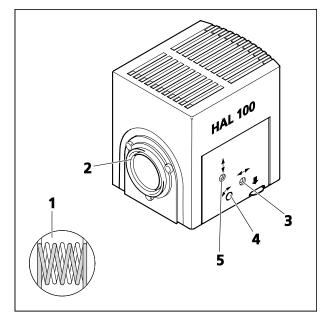
Fig. 3-38 Adjusting the HAL 100 halogen illuminator
