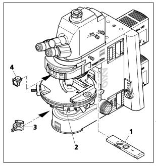
Fig. 4-122 Components for transmitted-light polarization
