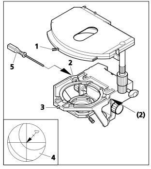
Fig. 3-53 Centering the rotary mechanical stage
