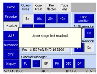
Fig. 4-28 Motorized focusing drive has reached the upper stage limit switch
