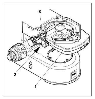
Fig. 3-11 Attaching the achromatic-aplanatic universal condenser, mot.
