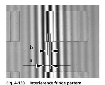
The values for a and b (see Fig. 4-133) are determined using the eyepiece reticle or the micrometer eyepiece.
