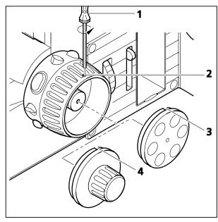
Fig. 3-19 Changing the fine-drive knob or fine-drive disk
