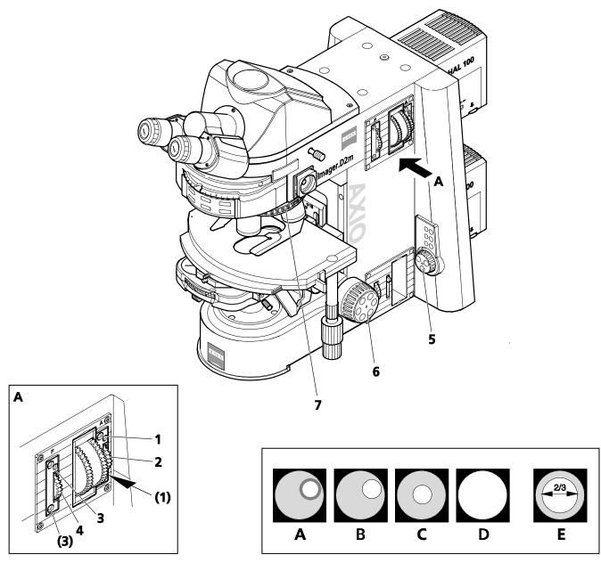
Fig. 4-128 Microscope settings on Axio Imager MAT in reflected-light brightfield
