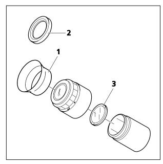
Fig. 3-5 Inserting the fold-over eyecups
