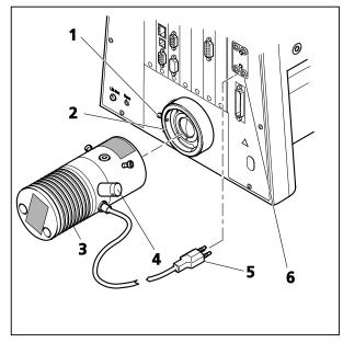
Fig. 3-42 Installing the attachment lamp VIS-LED
