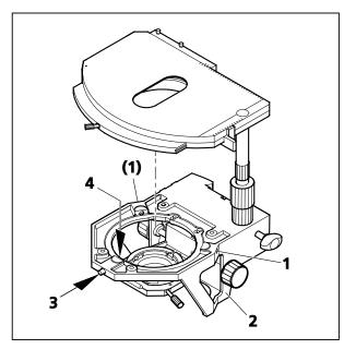
Fig. 3-52 Changing the rotary mechanical stage
