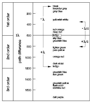
Fig. 4-124 Schematic diagram of the color charts according to Michel-Lévy
