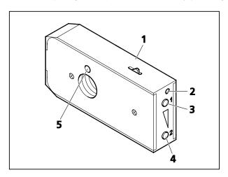
Fig. 4-6 Inserting/removing filter wheel 2x discrete mot.
