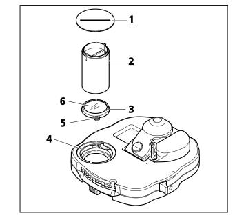
Fig. 3-12 Replacing the DIC prism
