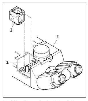
Fig. 4-14 Receptacles for P&C modules
