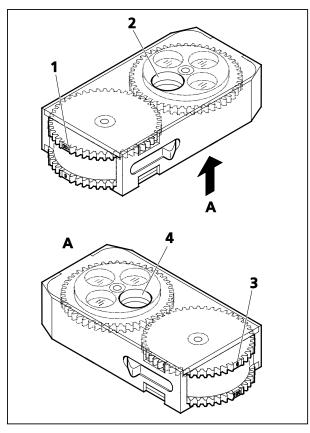
Fig. 3-20 Equipping 2-position filter wheel, manual
