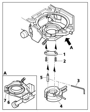
Fig. 3-59 Installing Polarizer D, fixed
