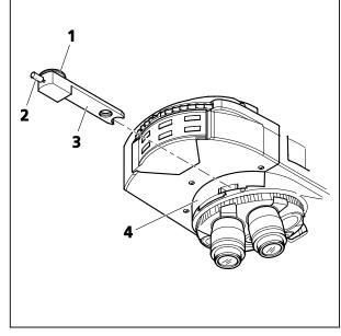
Fig. 4-129 6x20 compensator mount with 6x20 C-DIC slider
