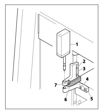
Fig. 3-31 Installing the focus linear sensor
