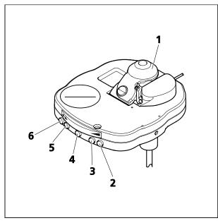
Fig. 4-8 Achromatic-aplanatic universal condenser, mot.
