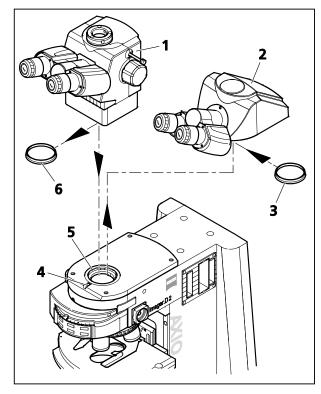
Fig. 3-2 Changing the binocular tube
