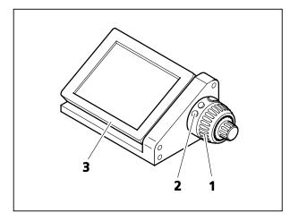
Fig. 4-18 Docking station with TFT display, pushbutton ring and focusing drive
