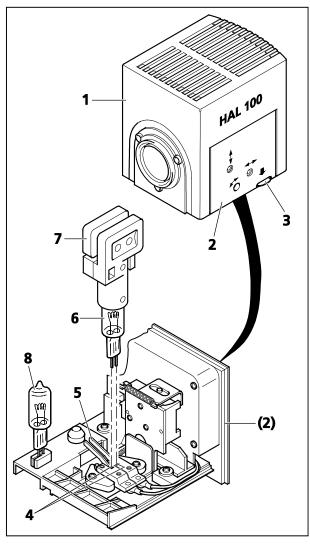
Fig. 3-39 Changing the halogen lamp
