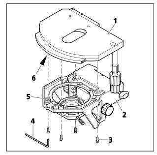
Fig. 3-51 Changing the fixed mechanical stage
