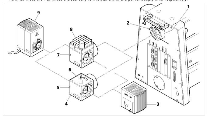
Fig. 3-48 Installing the switching mirror
