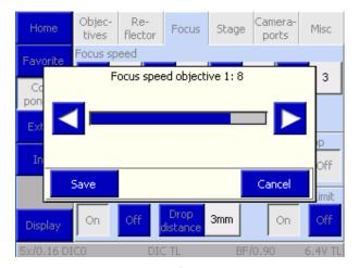
Fig. 4-67 Setting the focusing speed
