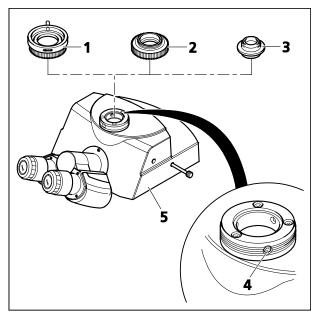
Fig. 3-8 Fitting components to the phototube
