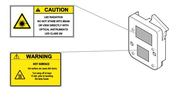
Fig. 1-3 Warning stickers on the underside of the LED illuminator
