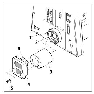
Fig. 3-40 Installing the LED illuminator
