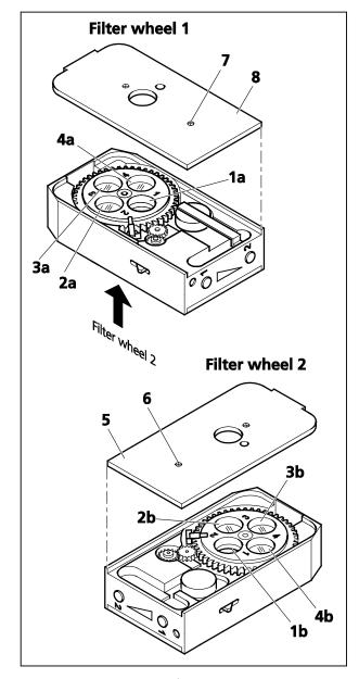
Fig. 3-21 Equipping filter wheel 2x, motorized (only for 428301-9901-000)
