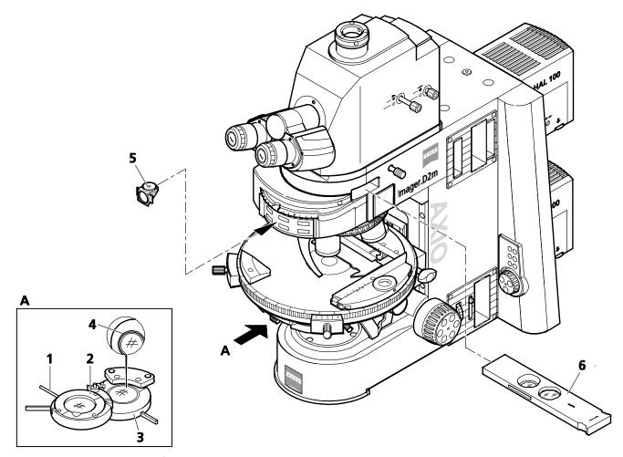
Fig. 4-125 Components for circular polarization contrast
