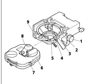
Fig. 3-10 Attaching the achromatic-aplanatic universal condenser
