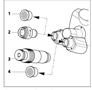
Fig. 3-4 Inserting eyepieces
