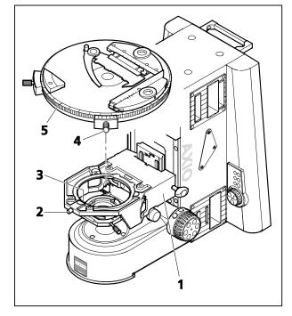
Fig. 3-56 Attaching rotary stage Pol
