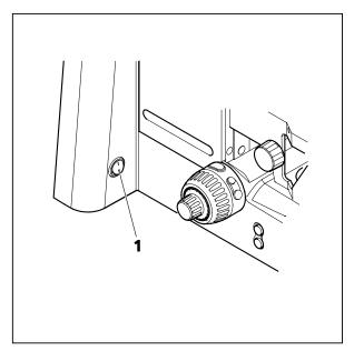
Fig. 4-9 Switching the manual microscope on/off
