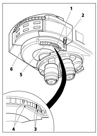
Fig. 4-130 4-position modulator turret
