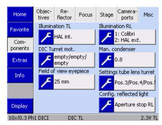
Fig. 4-76 Microscope -> Settings -> Components -> Misc(ellaneous)
