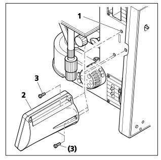
Fig. 3-29 Mounting the TFT display
