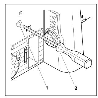
Fig. 3-28 Activating/deactivating the highperformance focus
