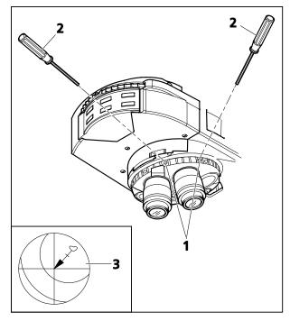
Fig. 3-58 Centering rotary stage and objectives
