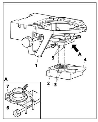
Fig. 3-41 Installing the LED illuminator
