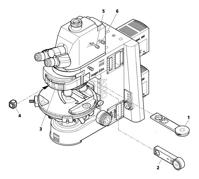
Fig. 4-135 Components for reflected-light polarization
