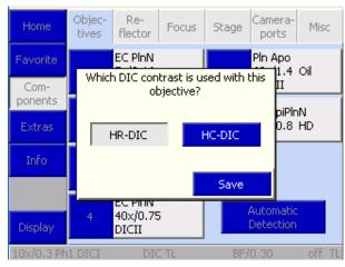
Fig. 4-59 Allocating the DIC slider
