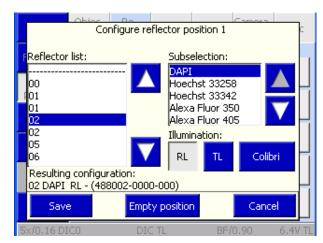
Fig. 4-63 Configuring the reflector position using Colibri
