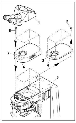
Fig. 3-3 Mounting the tube lens turret
