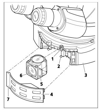
Fig. 3-22 Changing P&C reflector modules
