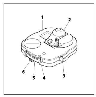
Fig. 4-4 Achromatic-aplanatic universal condenser 0.9 H D Ph DIC
