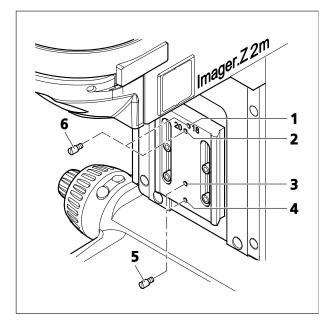
Fig. 3-16 Setting dovetail guide stops
